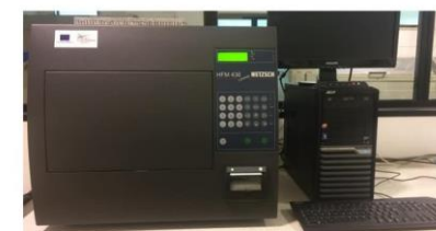
Figura 1 –NETZSCH heat flow meter HFM 436/0/1
